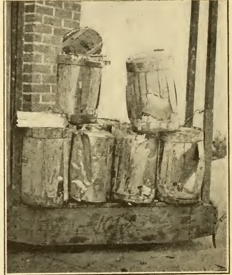
A truck-load of round wooden-jacketed cans just as they were received after shipment.
